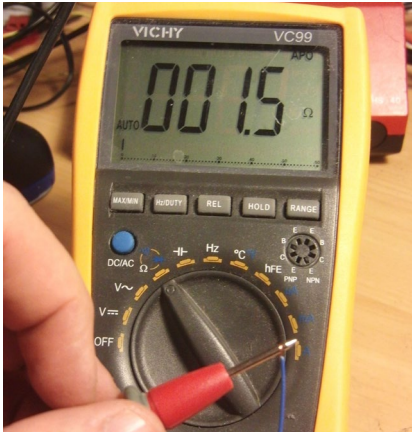
Image 3. A multimeter shows that the ends of the wire are connected.
